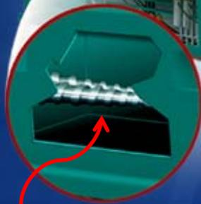
Screws Push Compound Through Extruder and Die
