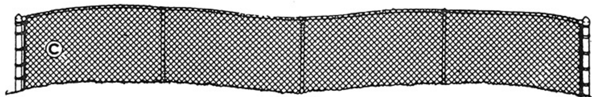
C Fence following grade
